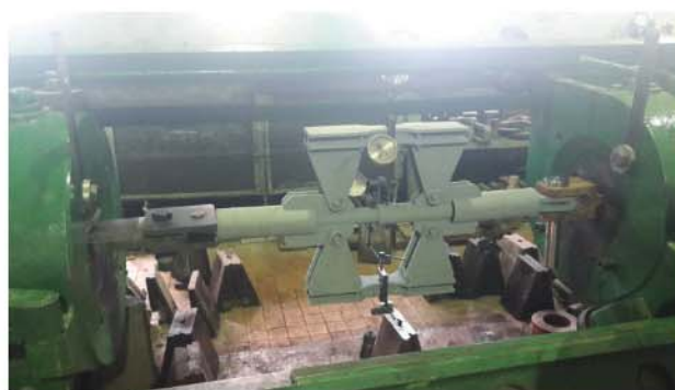
Figure 3. Full-scale experiment for axial damper
